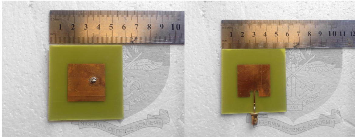
Figure 13a: Fabricated Patch with Coaxial feed method, 13b: Patch antenna with microstrip line feed method.
